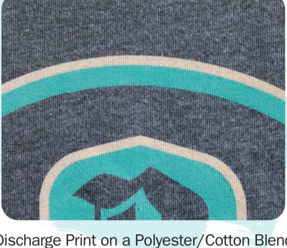
Discharge Print on a Polyester/Cotton Blend
